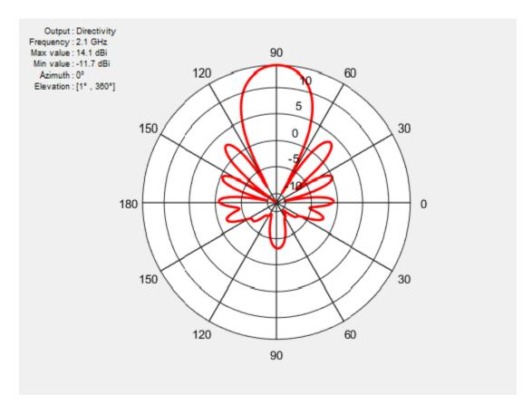
Half power beamwidth (HPBW) is the angular separation in which the magnitude of the radiation pattern decreases by 50% (or -3dB) from the peak of the main beam
