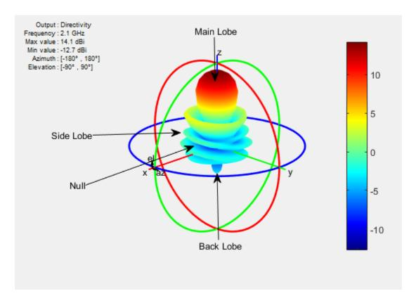
Use the pattern function to plot radiation pattern of any antenna in the Antenna Toolbox. By default, the function plots the directivity of the antenna. You can also plot the electric field and power pattern by using *Type* name-value pair argument of the pattern function.
