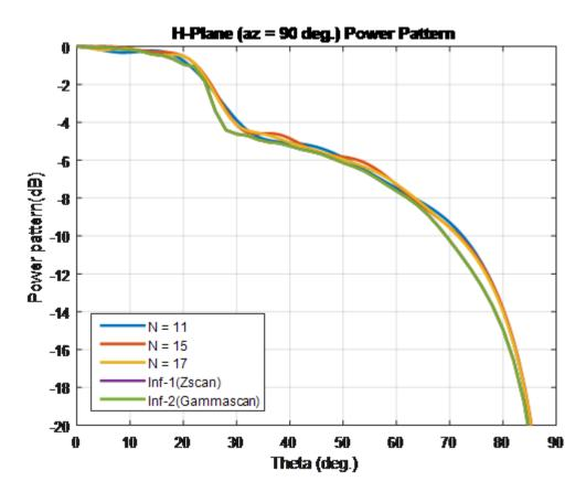
For finite arrays of size greater than 10 x 10, the scan element patterns in the E-, D-, and H-planes match the patterns of the infinite array scan element.
