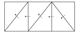
According to the method of images, the real and image electric currents are equal to each other in terms of magnitude. The parallel components are in opposite direction. The normal components are in the same direction.
