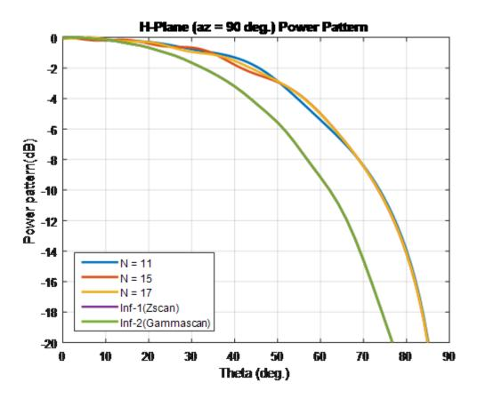
Case 2: Compare finite array and infinite array with unit cell of dimensions  $0.7\lambda \times 0.7\lambda$
