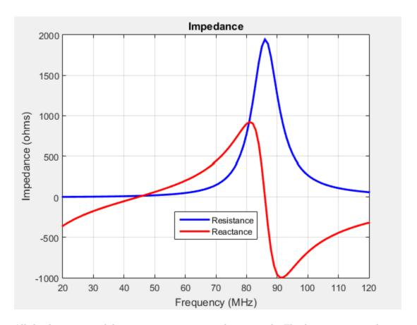
All the dimensions of this antenna are same as the monopole. The first resonance of the antenna is approximately  $45~\mathrm{MHz}$ . To view the accumulated charges on the top-hat monopole, use the <code>charge</code> function:
