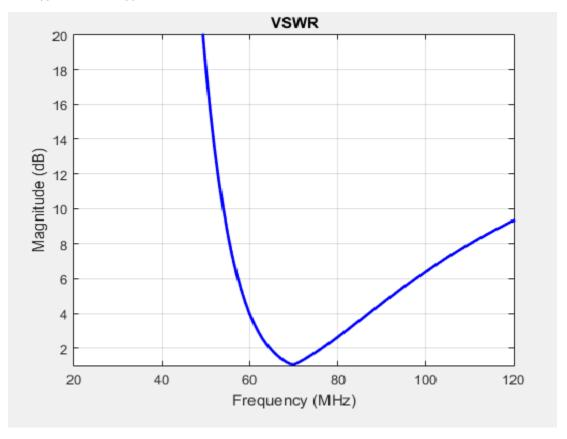
VSWR is scalar and contains no phase information. The value of VSWR lies between 1 and infinity. Antenna bandwidth is usually the frequency band over which the VSWR is less than approximately 2.
