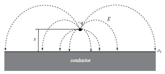
You can also apply this equivalence in reverse. Consider charges that are distance x apart from a conducting surface. You can replace the conducting surface with a set of image charges whose signs are opposite those of the original charge. Place these image charges at a distance x below the original conducting surface. This method eliminates the conducting plate, leaving only charges in unbound space. This equivalence is called the method of images.
