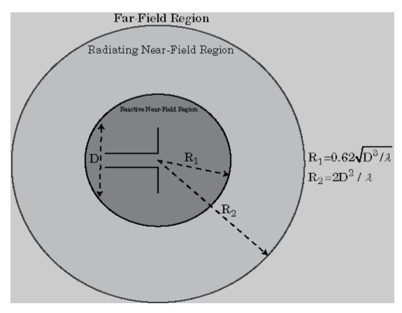
The region around an antenna is defined in many ways. The most used description is a 2- or 3-region model. The 2-region model uses the terms *near field* and the *far field* to identify specific dominant field mechanisms. The diagram is a representation of antenna fields and boundaries. The 3-field region splits the near field into a transition zone, where a weakly radiative mechanism is at work.
