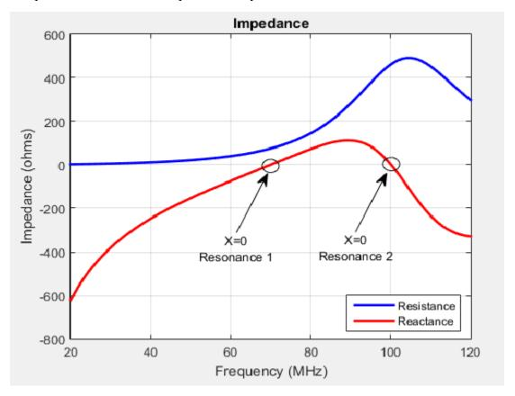
In the plot, the reactance values are negative, or capacitive, before the resonance. These values are positive or inductive after the resonance. This type of resonance is called series resonance. You can model this type of resonance using a series RLC circuit. If the
