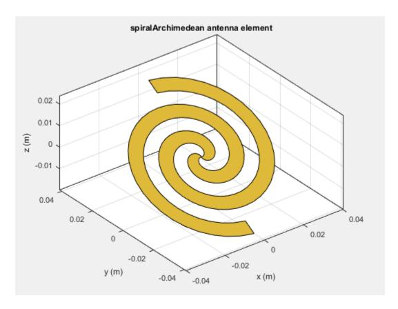
Use this spiral antenna to make a three-element linear array of tilted spirals.
