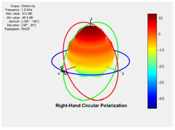
• Left-Hand circularly polarized (LHCP): The electric field vector is traced in the clockwise direction. To view the LHCP pattern of an antenna, use the pattern
